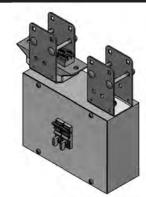
Breakered line-feed (up to 20 Amps) can be positioned anywhere on busSTRUT to reduce the length of homeruns. Features a 3 Pole Fitter that powers up to two 20A circuits; 40A max. Available in galvanized, powder coated white and black. Universal 120/277V. Mounts to both single and double-deck busSTRUT/20. Factory installed Circuit Breakers.
