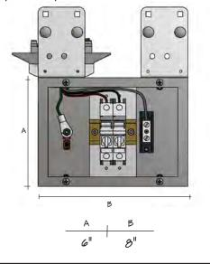
busSTRUT (single and double-deck) Product Voltage Amp Catalog Number LINE-FEED UNIVERSAL 20 P20-3-40-UNIV-CB20-(F) (BREAKERS) 120/277 Custom P20-3-40-UNIV-CBXX-(F)
