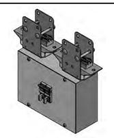
Breakered line-feed (up to 40 Amps) can be positioned anywhere on busSTRUT to reduce the length of homeruns. Features two 3 Pole Fitters that power up to two 40A circuits; 80A max. Available in galvanized, powder coated white and black. Universal 120/277V. Mounts to both single and double-deck busSTRUT/40. Factory installed Circuit Breakers.
