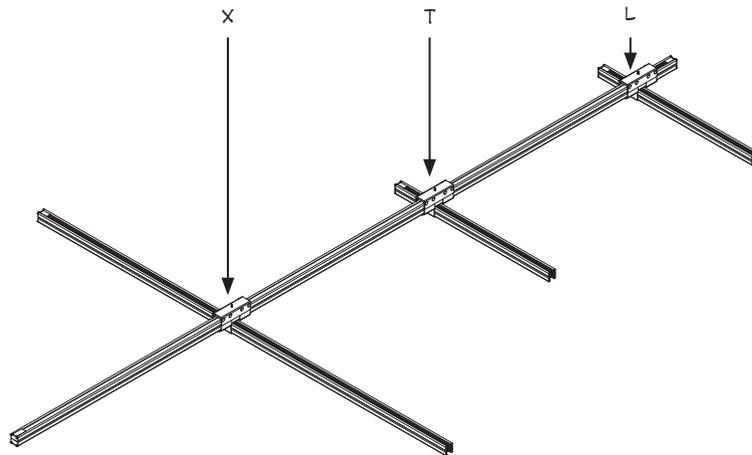
Crossovers provide the mechanical connection for building runs, rows, and grids. One universal crossover serves as an X,T, or an L intercept. The TWO over TWO crossover is used when one double-deck length of busSTRUT intersects another double-deck length of busSTRUT.
