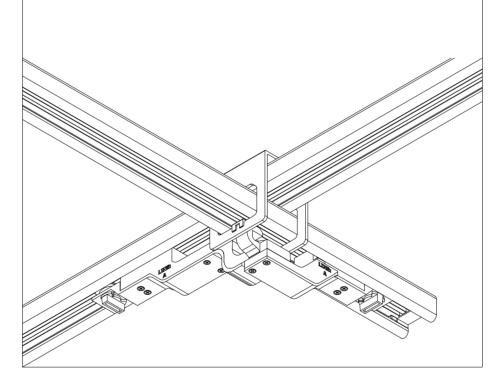
Seat the jumper into the busSTRUT by squeezing tightly on one side and turning the knob. Then, turn the other knob to complete the circuit.
